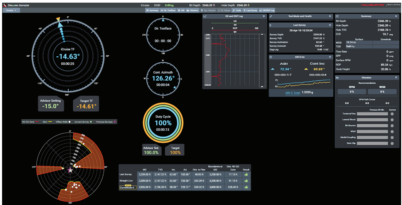
Fig. 3. The drilling advisor screen, showing real-time survey data and steering recommendations.
