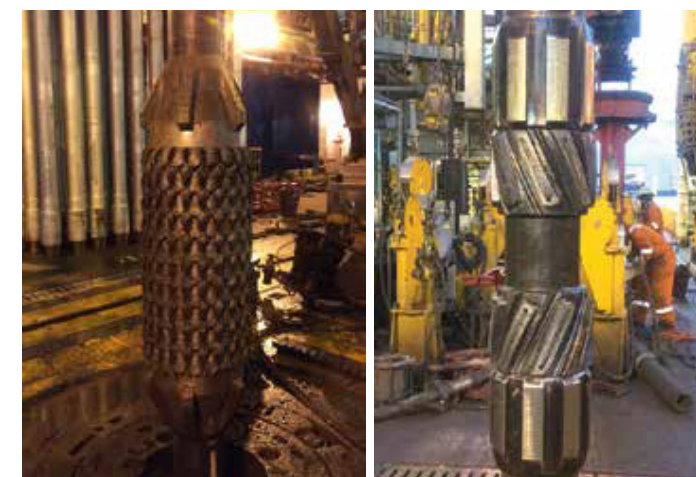
Mag Tech® riser magnet recovers 97.43 pounds of well debris.
